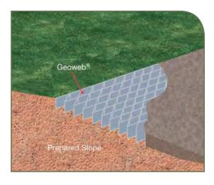
The Geoweb® system is the most advanced soil stabilization technology available on the market today. Initially developed by the US army to allow trafficking of heavy vehicles over very soft ground.
